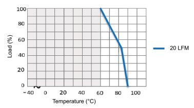
The derating curve was measured at 24 V input
